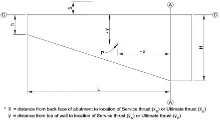
Figure 3 - Horizontal Load Geometry
